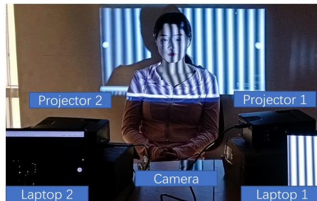
Figure 4. The physical settings of the phase superposition attack. The adversary uses an additional projector to add noises to the original fringe images for 3D reconstructions.
